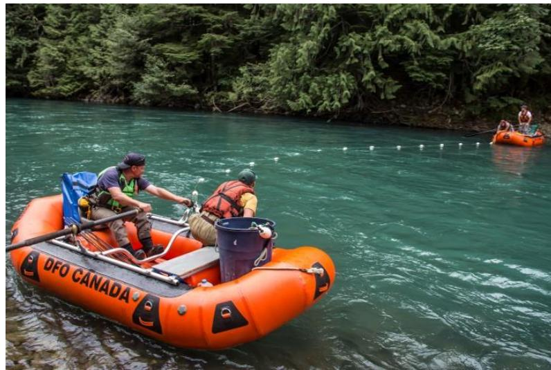
Step 4 –Near the tail out, raft 1 will start to row back across the river. At the same time, raft 2 will find a safe spot for a crew member to jump out and anchor the net.
